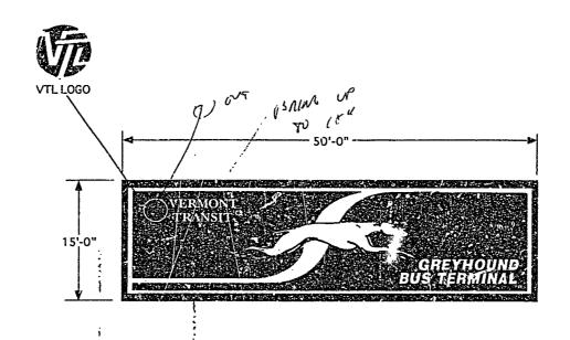
B. MANUFACTURE AND INSTALL 1) SINGLE-FACED, NON-ILLUMINATED SIGN BOX WITH A FLEX FACE AS SHOWN. OPTION:—TIFFAN-BOARDS.
