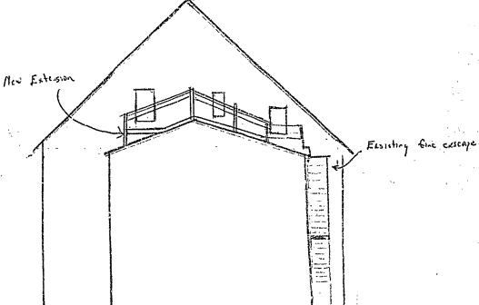
Proposed extention of fire existage in blue 2x4 platform with 3/4 decking with 4x4 post and 2x11 ruils connecting to existing fire existing
