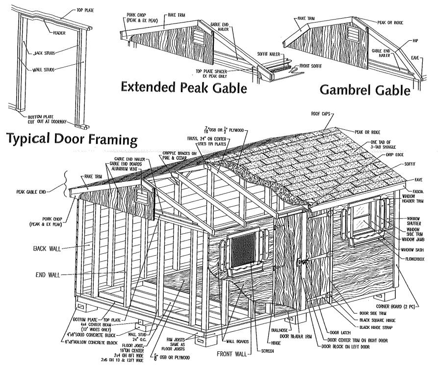
**Cutaway of Pine Shed with Peak Roof**
