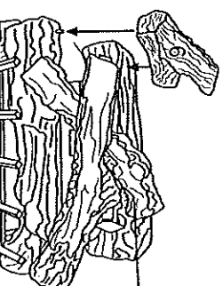
Figure 50 - Installing Log No. 6
