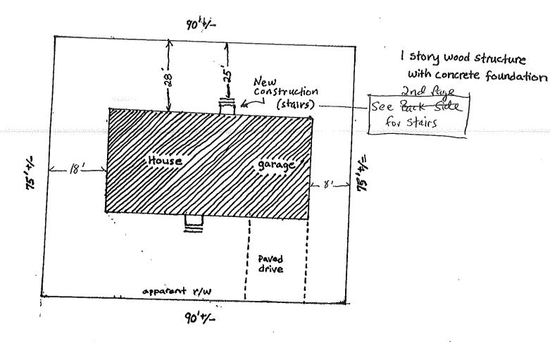
Note: Previous owners of property built a deck without a permit that was in violation of set back (25'). The deck was removed and the new owners (Borelli's) are re-attaching the stairs, that were part of the deck, back to the house.
