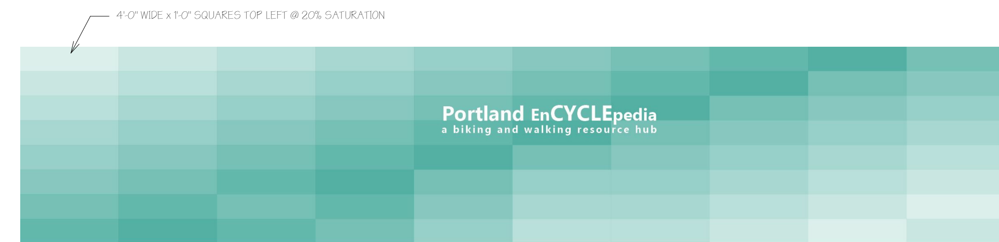
PAINTING PATTERN - 4x8 SHEETS OF PLYWOOD MARKED IN 1'-0" INCREMENTS VERTICALLY, 10% COLOR SATURATION DIFFERENTIAL BTW 20% AND 100% - UPPER LEFT HAND CORNER = 20%
