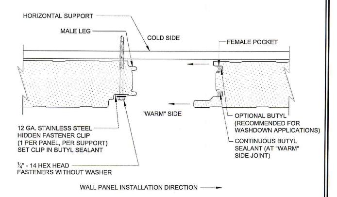
NOTE: FILL FEMALE POCKET(S) 3/4 FULL WITH SEALANT TO PROVIDE PROPER AIR/WATER SEAL
