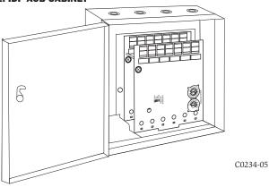
The front SK-Relay-6 module positions of each chassis are offset below the rear SK-Relay-6 module positions so that all of the status indicators are visible. For cabinet dimensions refer to IDP-ACB instruction manual.
