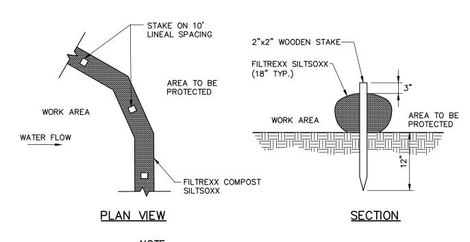
WHEN STAKING IS NOT POSSIBLE, HEAVY CONCRETE BLOCKS SHALL BE USED BEHIND THE SEDIMENT CONTROL TO HELP STABILIZE DURING RAINFALL/RUNOFF EVENTS.
