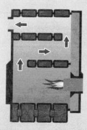
The three pass design of the Quatech boiler insures a more efficient system by have the flue gases travel a longer path. The flue gases can then heat a larger surface area and reduce heat loss up the chimney saving you money.
