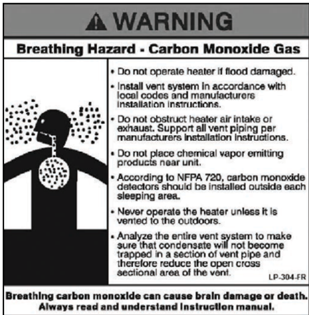
Figure 5 - CO Warning Label
