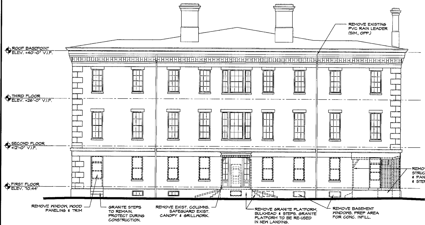
3 EXISTING EAST ELEVATION A4.1 1/8" = 1'-0"
