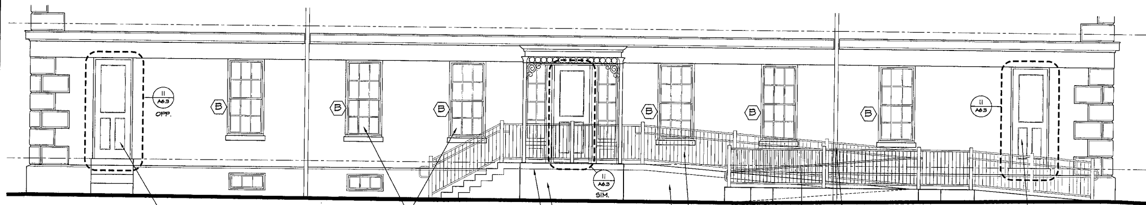
3 PROPOSED EAST ELEVATION - ADA ENTRY RAMP A4.3 1/4" = 1'-0"
