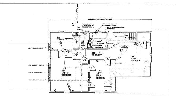
SECOND FLOOR PLAN RENOVATIONS 1 A-3 SCALE: 1/4" = 1"-0"
