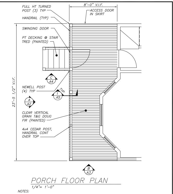
1. ALL COMPONENTS TO BE PRIMED ALL SIDES PRIOR TO ASSEMBLY USING OWNER SUPPLIED PRIMER INCLUDING TOP AND BOTTOM HANDRAILS, BALUSTERS, PORCH POSTS, NEWELL POSTS, AND DECKING.
