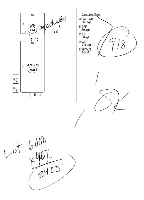
The Home Depot # 2401 245 RIVERSIDE STREET, PORTLAND, ME 04103 (207) 761-0600 Wed Jun 22 11:16:37 2005 BOB EVEREST **DECK** 216796 Construction Specifications deck 1: Construction Method = Beam on Top of Post Footing Type = Pier In-Ground Live Load = 40 Dead Load = 10 Decking Spacing = 0 1/4" Joist Spacing = 16" Beam Spacing = 167" Post Spacing = 167
