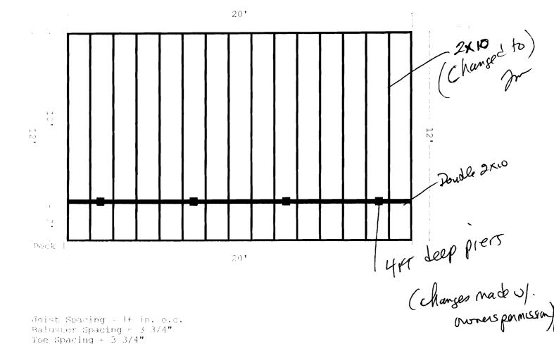
Joist Spacing > 16 in. o.c. Baluster Spacing = 3 3/4" Toe Spacing = 3 3/4" Railing Height = 36"
