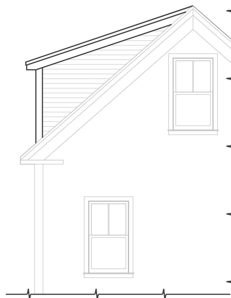
FRONT ELEVATION SHOWING NEW DORMER
