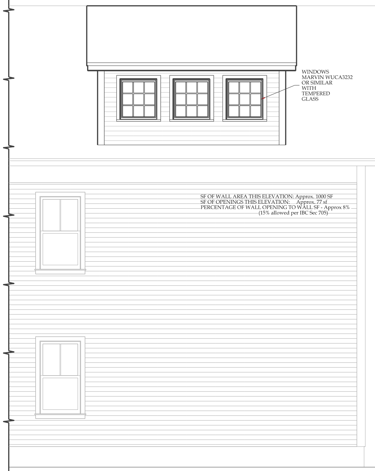
LEFT SIDE ELEVATION SHOWING NEW DORMER
