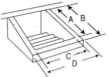
Write the four door measurements, A,B, and C, D, in space below. Using these measurements and the chart, choose the right door size. Not sure?? Ask your Gordon dealer for Help.
