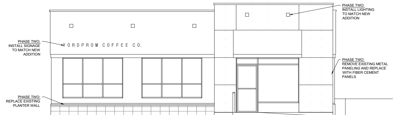
13 NORTH ELEVATION - EXISTING BUILDING PHASE TWO 1/4" = 1'-0"
