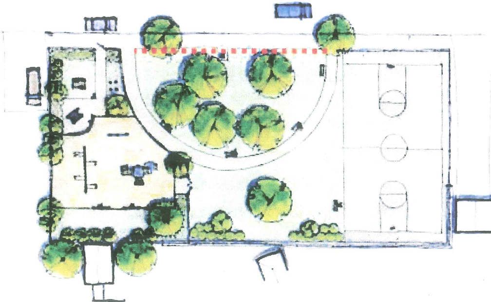
TAYLOR STREET FENCE: Existing 4' tall chain-link fencing along Taylor Street will be removed as part of the Taylor Street Park Improvements project (Above image: orange dotted line).
