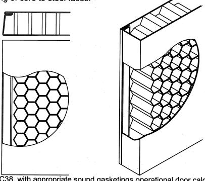
Inoperable panel STC38, with appropriate sound gasketings operational door calculated STC of 33. Added stiffener, full height, in middle of door when over 3'0" wide.
