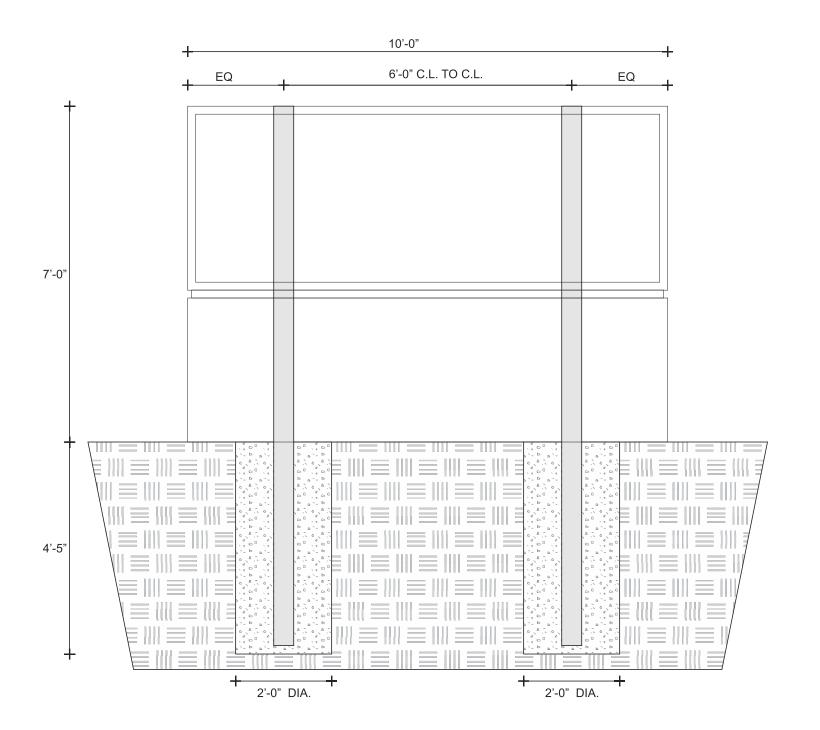
**SIGN ELEVATION - DETAIL** SCALE: 1/2" = 1'-0"
