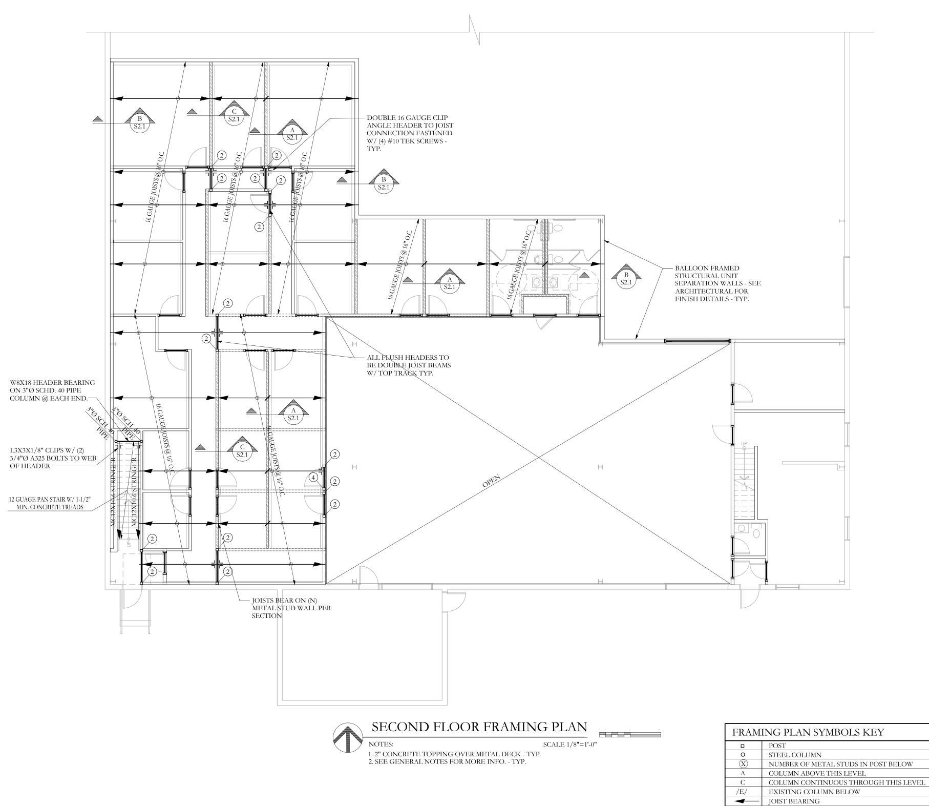
← CONTINUOUS JOIST WITH INTERMEDIATE BEARING ► FLUSH FRAMED JOIST BEARING WITH HANGER METAL STUD BEARING WALL BELOW SHEAR WALL NUMBER OF TRIM STUDS UNDER HEADER NUMBER OF KING STUDS ADJACENT TO HEADER
