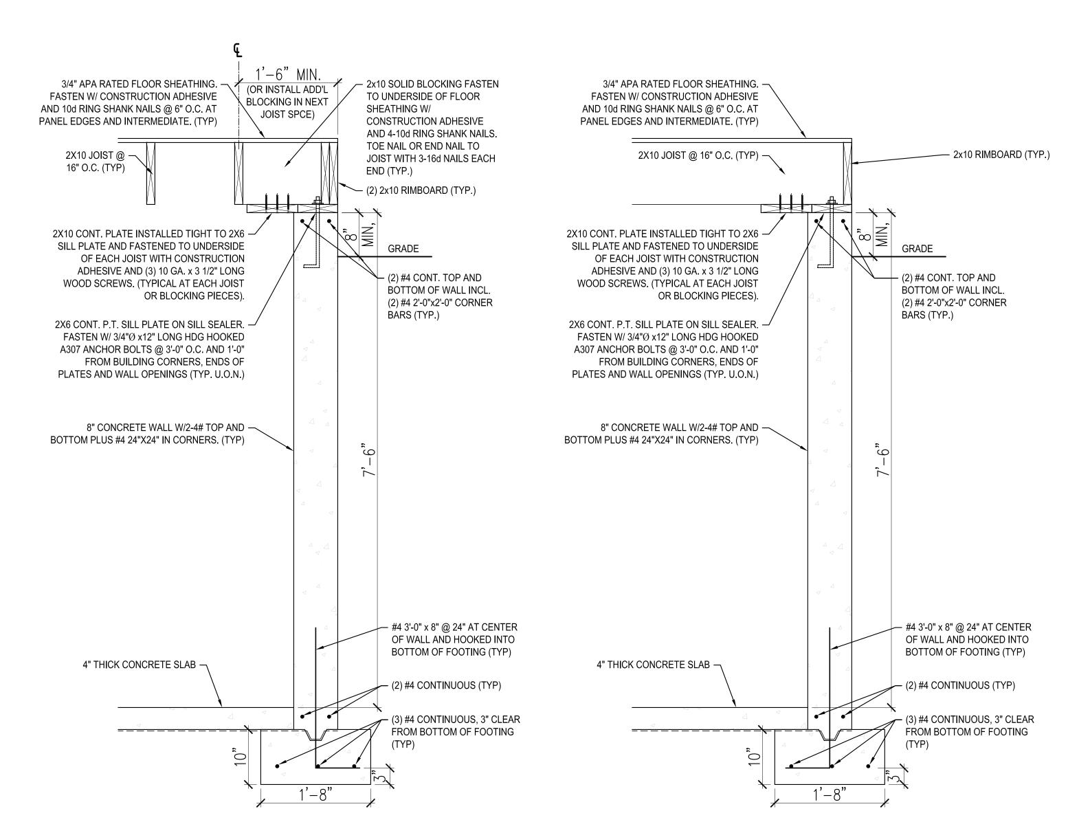
A FOUNDATION/FLOOR FRAMING SECTION (JOISTS PARALLEL TO WALL)
