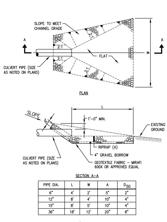
RIPRAP INLET/OUTLET PROTECTION SCALE: N.T.S.
