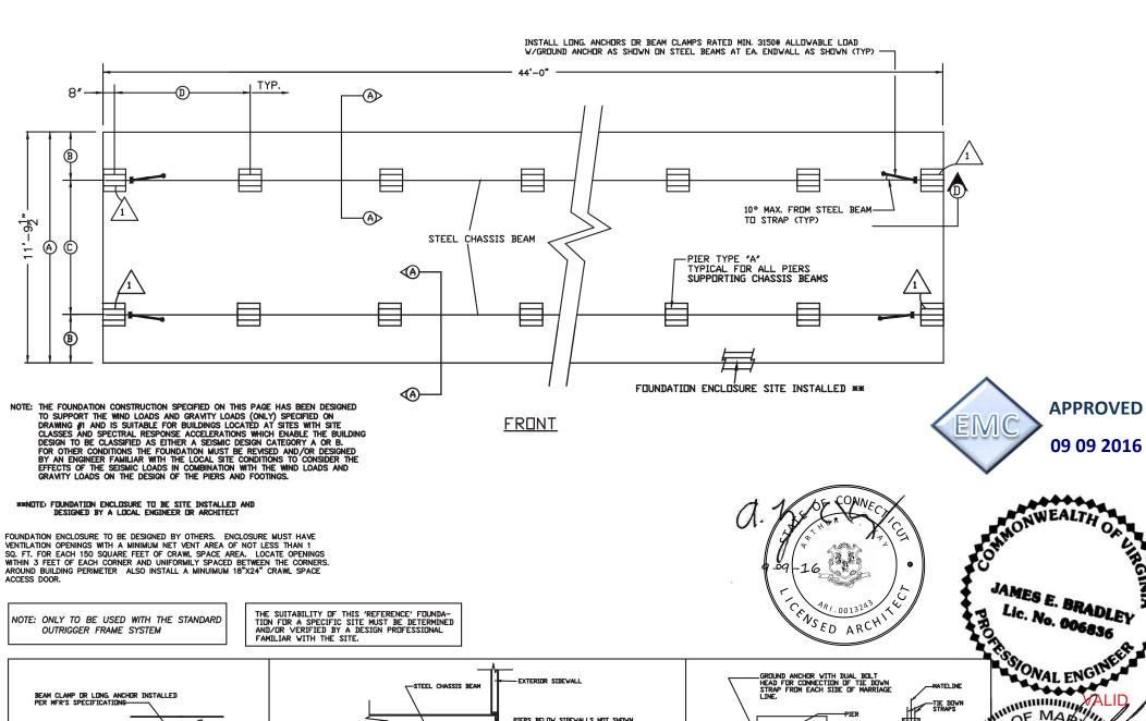
BEAM CLAMP OR LONG. ANCHOR INSTALLED PER MFR'S SPECIFICATIONS PIERS BELOW SIDEWALLS NOT SHOWN FRAME TIE-DOWN STRAP AND GROUND ANCHOR AT 7'-0" (LOCATE FIRST ANCHOR VITHIN 2' FROM EACH END OF FLOOR) SECTION B-B SECTION D-D PLAN VIEW OF VERTICAL TIE DOWN STRAP AT MARRIAGE FOOTING MUST EXTEND BELOW FROST LINE SECTION C-C SECTION A-A
