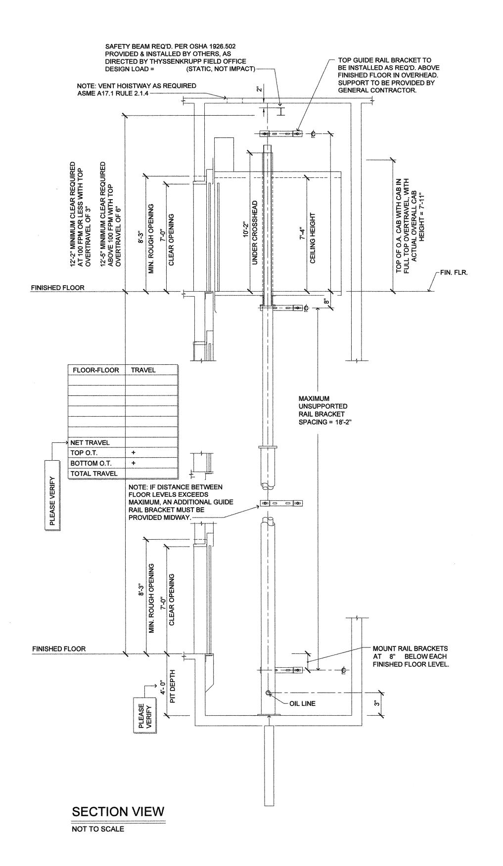
VERIFY HOISTWAY DIMENSIONS WITH MANUFACTURE PRIOR TO POURING ELEVATOR PIT
