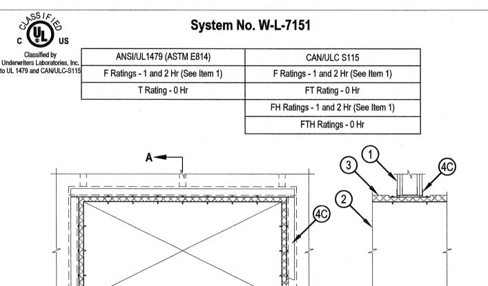
1. Wall Assembly — The fire-rated gypsum board/stud wall assembly shall be constructed of the materials and in the manner specified in the individual U300, U400, V400 or W400 Series Wall and Partition Designs in the Fire Resistance Directory and shall include the following
