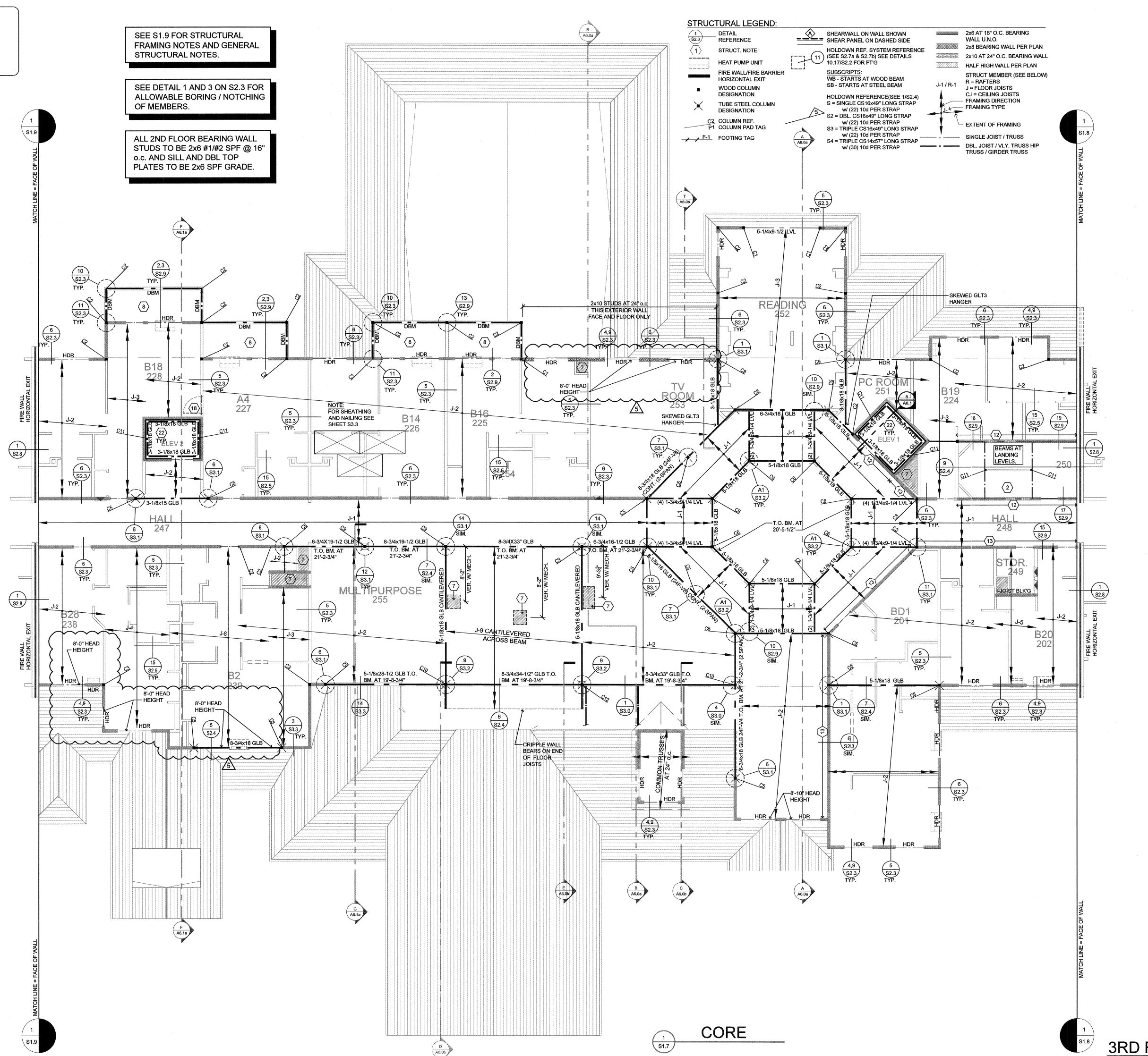
**COLUMN SCHEDULE** MATERIAL BASEPLATE COL SPF #1/#2 OR BETTER DFL #2 C1 SPF #1/#2 OR BETTER C2 SPF #1/#2 OR BETTER C3 5 **\** 6x8 3-1/2x3-1/2x1/4" 9-1/2"x0'-91/2x3/4" C4 ASTM A500 ASTM A500 10"x0'-10"x3/4" C5 4x4x1/4" C6 ASTM A500 4x4x5/16" 10"x0'-10"x3/4" ASTM A500 10"x0'-10"x3/4" C7 4x4x3/8" C8 ASTM A500 5x5x3/8" 11"x0'-11"x3/4" C9 ASTM A500 5x5x1/4" 11"x0'-11"x3/4" 12"x12"x3/4" C10 ASTM A500 6x6x5/16" C11 C12 ASTM A500 8x8x1/4" 14"x14"x3/4"
