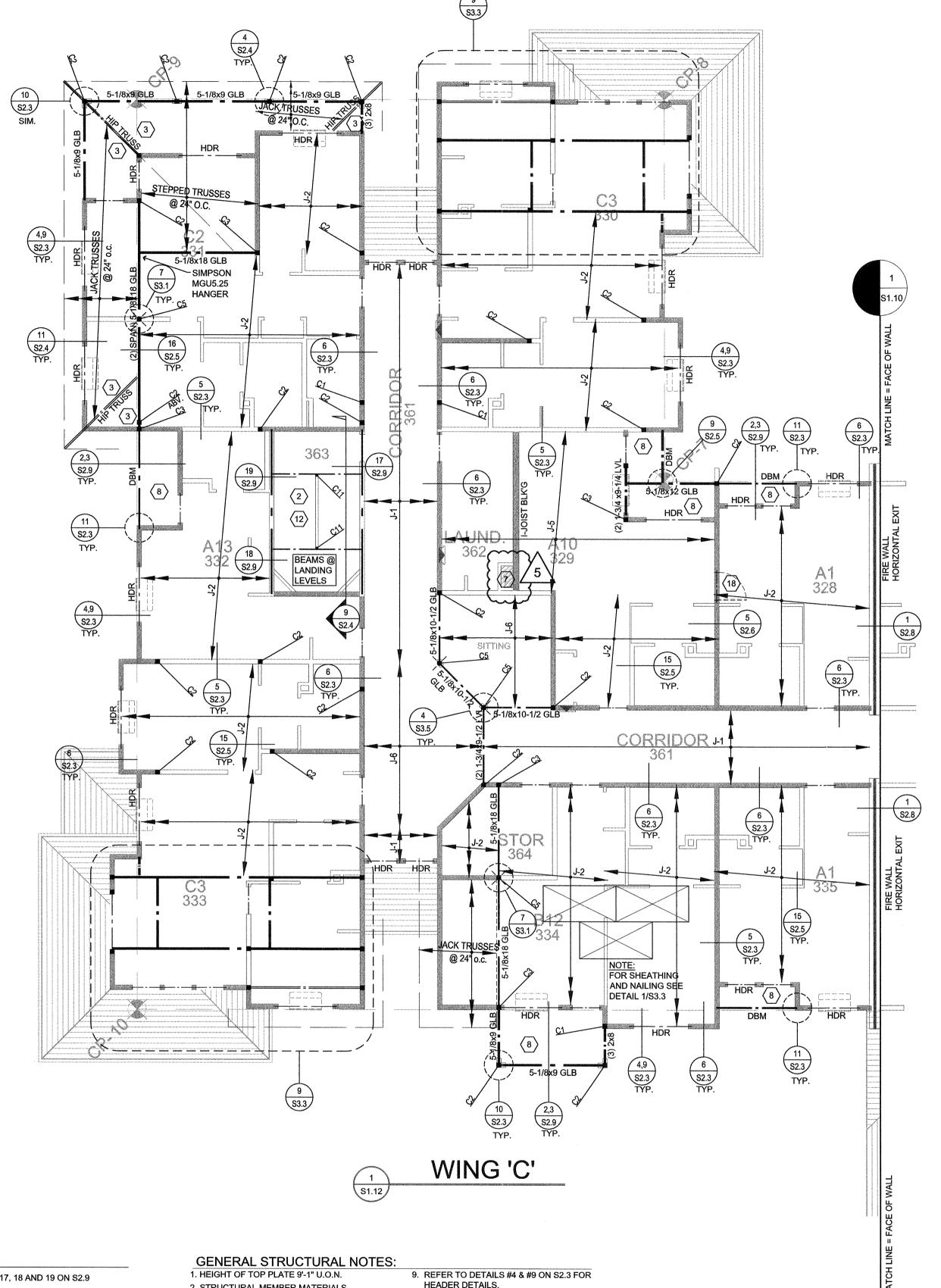
F-1 FOOTING TAG S4 = TRIPLE CS14x57" LONG STRAP ====== DBL. JOIST / VLY. TRUSS HIP w/ (30) 10d PER STRAP
