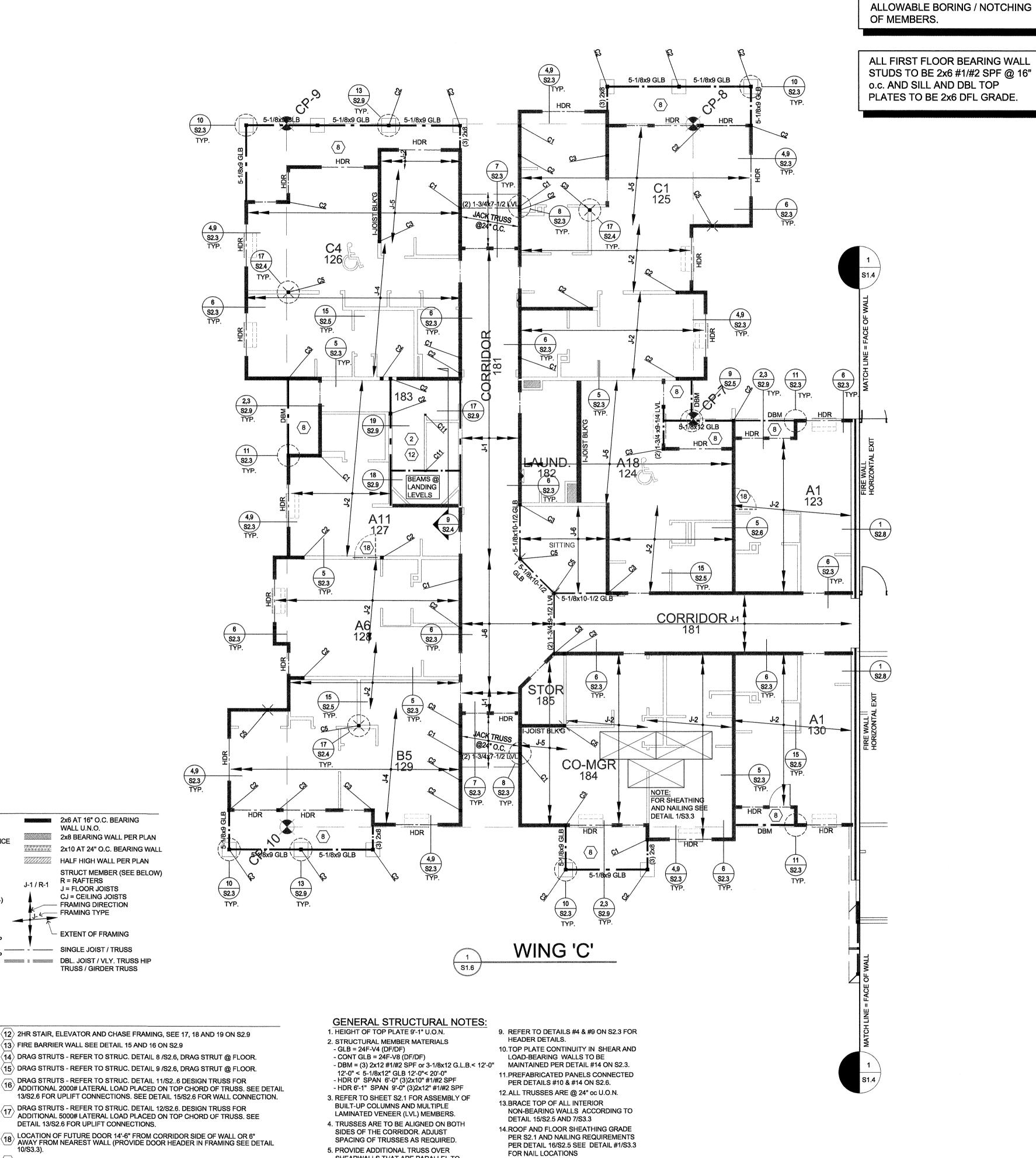
COLUMN SCHEDULE COL MATERIAL SIZE BASEPLATE SPF #1/#2 OR BETTER DFL #2 SPF #1/#2 OR BETTER (3) 2x6 C2 (4) 2x6 C3 C4 ASTM A500 3-1/2x3-1/2x1/4" 9-1/2"x0'-91/2x3/4' C5 ASTM A500 4x4x1/4" 10"x0'-10"x3/4" C6 ASTM A500 4x4x5/16" 10"x0'-10"x3/4" C7 ASTM A500 4x4x3/8" 10"x0'-10"x3/4" C8 ASTM A500 5x5x3/8" 11"x0'-11"x3/4" C9 ASTM A500 5x5x1/4" 11"x0'-11"x3/4" C10 ASTM A500 6x6x5/16" 12"x12"x3/4" C11 C12 ASTM A500 8x8x1/4" 14"x14"x3/4"
