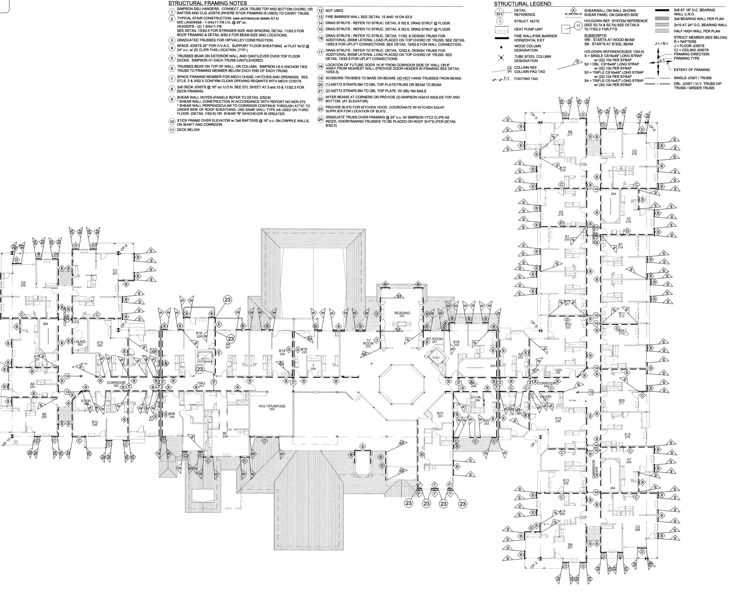
1. 3x STUDS AT ADJOINING PLY'WD PANEL EDGES. 2. 3x STUDS AND SILL PLATES. STAGGER PLY'WD PANEL EDGES. 3. 3x DF/L STUDS AND SILL PLATES. STAGGER PLY'WD PANEL EDGES.
