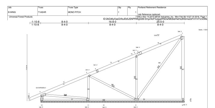
0-7-4 Plate Offsets (X,Y)-- [2:0-5-0,0-2-4], [7:0-2-0,0-2-4], [8:0-3-0,0-1-0], [11:0-2-8,0-3-0] LOADING (psf) SPACING-2-0-0 CSI. DEFL. (loc) I/defl L/d **PLATES GRIP** 40 n TC BC WB 0.00 197/144 Plate Grip DOL 1.15 0.80 Vert(LL) 180 MT20 n/r (Roof Snow=40.0) Lumber DOL 1.15 0.56 Vert(TL) 0.00 80 MT20HS 148/108 n/r TCDL 7.0 Rep Stress Incr NO 0.64 Horz(TL) -0.02 n/a n/a
