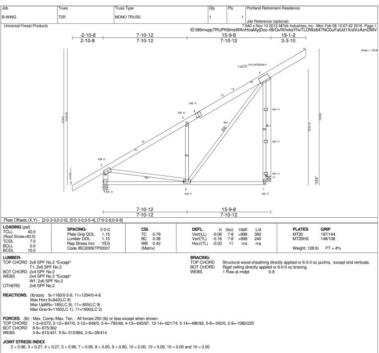
1) Wind: ASCE 7-05; 100mph; TCDL=4.2psf; BCDL=5.0psf; h=58ft; B=44ft; L=50ft; eave=4ft; Cat. II; Exp B; Kd 1.00; enclosed; MWFRS (all heights); cantilever left exposed; end vertical left exposed; Lumber DOL=1.60 plate grip DOL=1.60
