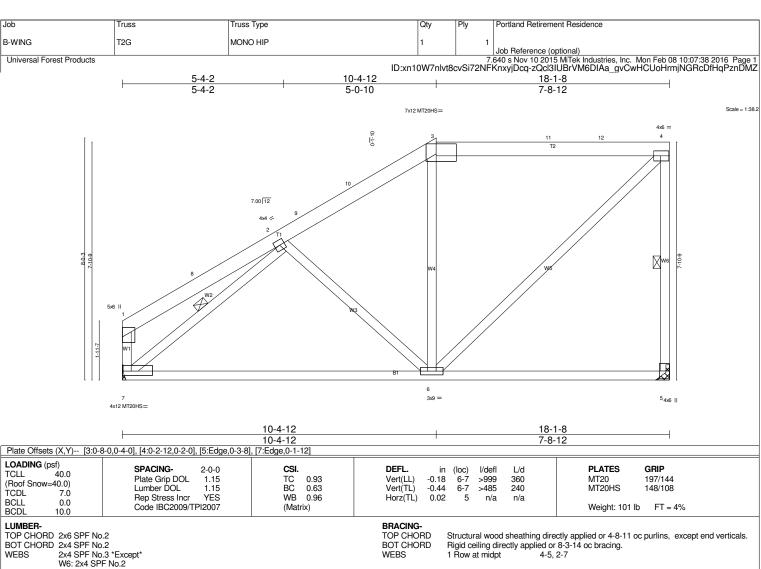
REACTIONS. (lb/size) 5=1017/Mechanical, 7=1017/Mechanical Max Horz 7=327(LC 9)
