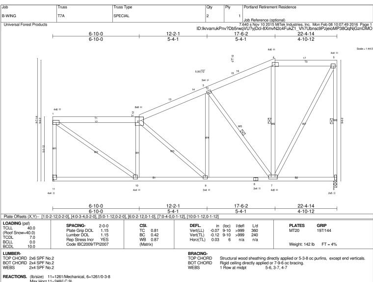
Max Horz 11=248(LC 9) Max Uplift11=-334(LC 9), 6=-489(LC 9) Max Grav 11=1333(LC 17), 6=1290(LC 18)
