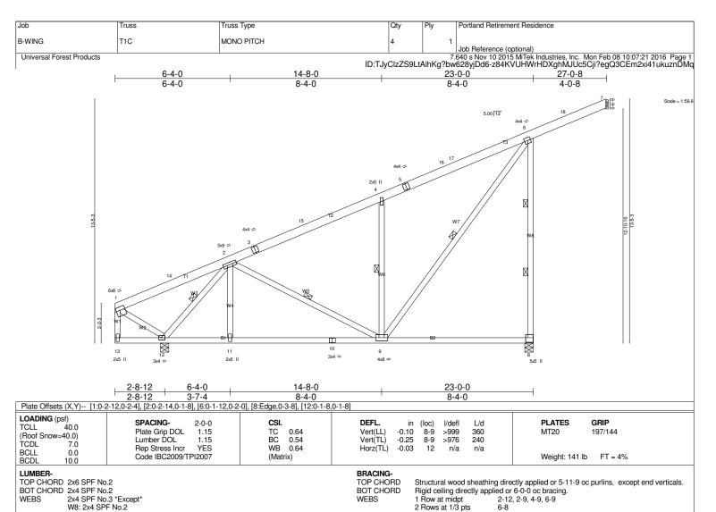
**REACTIONS.** (lb/size) 7=-0/Mechanical, 8=1439/0-5-8, 12=1533/0-5-8 Max Horz 7=-690(LC 22), 8=690(LC 22) Max Uplift8=-716(LC 9), 12=-322(LC 9) Max Grav 8=1833(LC 2), 12=1632(LC 2)
