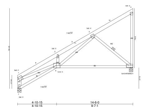
Plate Offsets (X,Y)-- [1:0-1-8,0-2-8], [3:0-2-4,0-2-4], [4:Edge,0-3-8], [5:Edge,0-2-12], [6:0-5-4,Edge] LOADING (psf) SPACING-2-0-0 CSI. **DEFL** in (loc) I/defl L/d **PLATES** GRIP TCLL 40 n TC BC WB Plate Grip DOL -0.21 360 197/144 1.15 0.88 Vert(LL) 5-6 >814 MT20 (Roof Snow=40.0) Lumber DOL 1.15 0.59 Vert(TL) -0.54 5-6 >315 240 MT20HS 148/108 TCDL 7.0 Rep Stress Incr YES 1.00 Horz(TL) 0.14 5 n/a BCLL Code IBC2009/TPI2007 (Matrix) Weight: 79 lb FT = 4%**BCDL** 10.0
