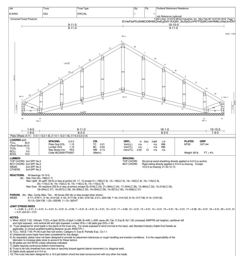
11) Provide mechanical connection (by others) of truss to bearing plate capable of withstanding 100 lb uplift at joint(s) 22, 17, 12 except (jt=lb) 21=195, 13=195, 18=102, 19=116, 20=110, 16=102, 15=116, 14=110.
