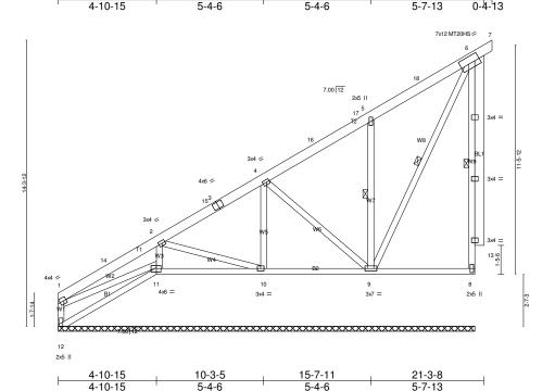
Plate Offsets (X,Y)-- [1:0-1-4,0-2-0], [2:0-1-12,0-1-8], [4:0-1-12,0-1-8], [6:0-5-0,0-4-0], [11:0-2-12,0-2-4] LOADING (psf) SPACING-2-0-0 CSI. DEFL. in (loc) I/defl L/d **PLATES** GRIP TCLL 40 n TC BC WB Plate Grip DOL -0.00 180 197/144 1.15 0.48 Vert(LL) MT20 6-7 n/r (Roof Snow=40.0) Lumber DOL 1.15 0.18 Vert(TL) -0.00 6-7 80 MT20HS 148/108 n/r TCDL 7.0 Rep Stress Incr YES 0.45 Horz(TL) -0.01 8 n/a n/a **BCLL** Code IBC2009/TPI2007 (Matrix) Weight: 147 lb FT = 4%
