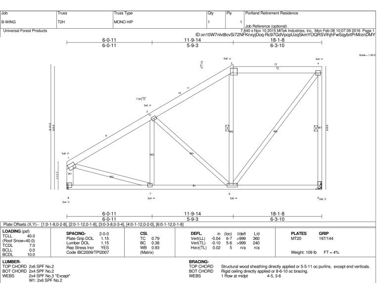
**REACTIONS.** (lb/size) 5=1012/Mechanical, 8=1012/Mechanical Max Horz 8=371(LC 9)
