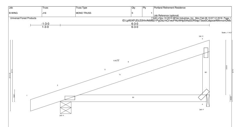
Plate Offsets (X,Y)-- [4:0-2-7,0-0-9] LOADING (psf) SPACING-2-0-0 CSI. DEFL. in (loc) I/defl **PLATES GRIP** 40 n TC BC WB Plate Grip DOL 1.15 0.84 Vert(LL) 0.11 >670 360 MT20 197/144 (Roof Snow=40.0) Lumber DOL 1.15 0.41 Vert(TL) -0.18 2-4 >395 240 TCDL 7.0 Rep Stress Incr NO 0.00 Horz(TL) 0.00 n/a Code IBC2009/TPI2007 (Matrix) Weight: 23 lb FT = 4% **BCDL** 10.0
