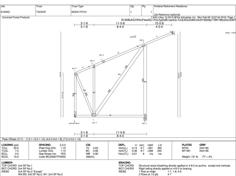
**REACTIONS.** (lb/size) 5=-0/Mechanical, 8=510/Mechanical, 6=535/0-5-8 Max Horz 5=-728(LC 35), 6=728(LC 35)
