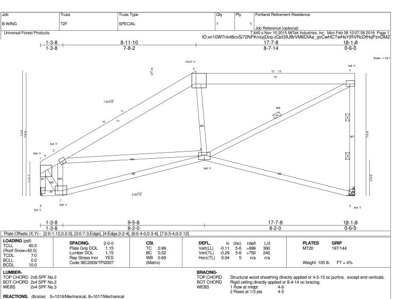
Max Horz 8=282(LC 9) Max Uplift5=-396(LC 9), 8=-268(LC 9) Max Grav 5=1339(LC 13), 8=1328(LC 14)
