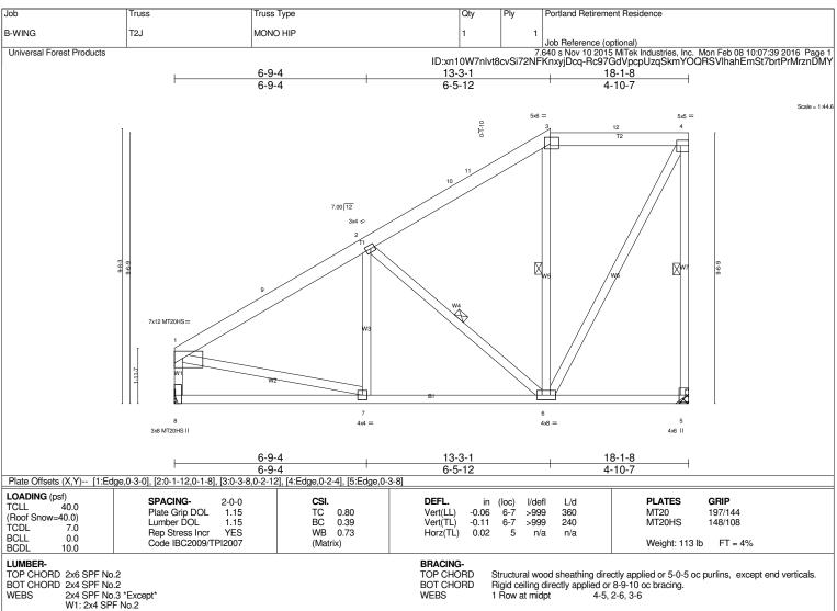
**REACTIONS.** (lb/size) 5=1017/Mechanical, 8=1017/Mechanical Max Horz 8=466(LC 8)
