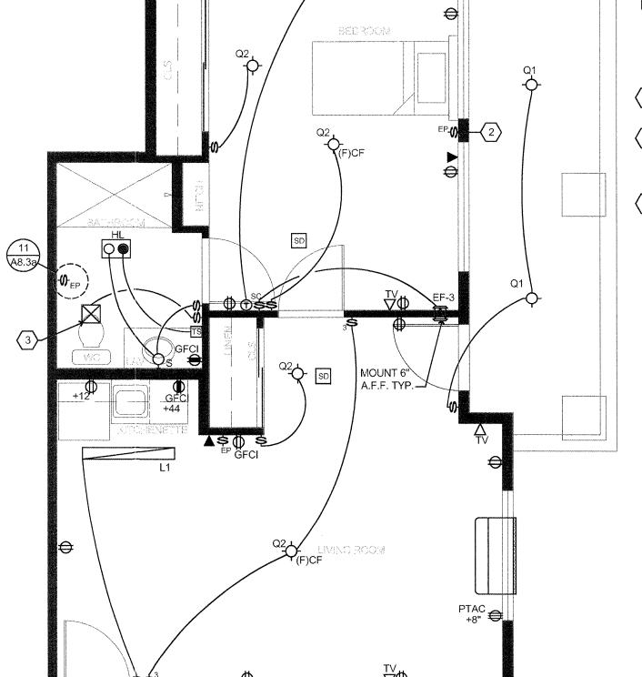
4. REFER TO ELECTRICAL DETAILS ON SHEET E2.2b. 5. INSTALL G.F.C.I. RECEPTACLE IN UNIT BATHROOMS AND AT BAR. RECEPTACLES WITHIN 6' OF SINK EDGE SHALL BE G.F.C.I PROTECTED.
