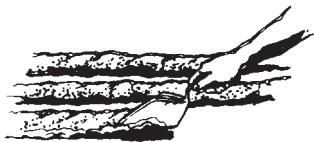
Figure 21 Placing Mortar for Hearthstone Installation
