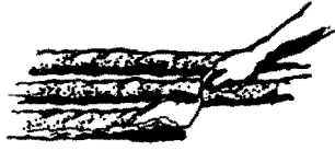
Figure 21 Placing Mortar for Hearthstone Installation
