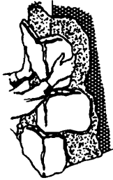
Figure 11 Applying corners - alternating long and short legs in the opposite directions
