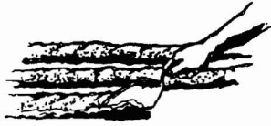
Figure 21 Placing Mortar for Hearthstone Installation
