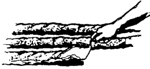
Figure 21 Placing Mortar for Hearthstone Installation
