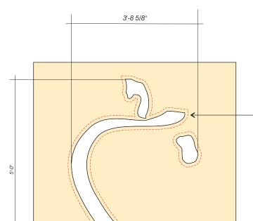
RED TRESPA BACK UP PANEL (BEST MATCH TO PMS #187 C) SURFACE: APPLY 3M HIGHLIGHTER FILM
