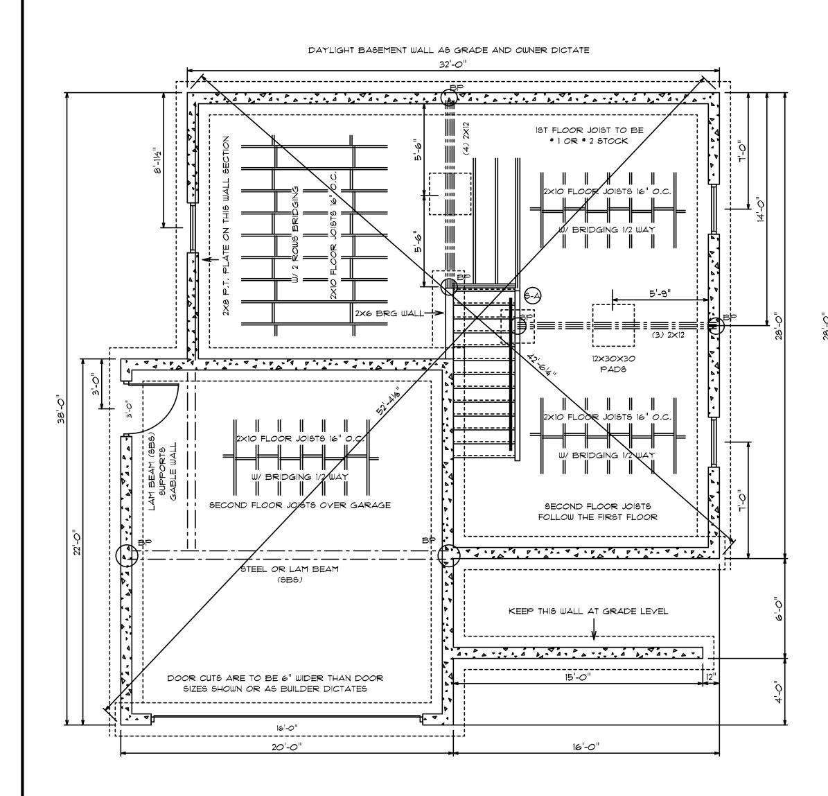
THE FOUNDATION, FOOTINGS, FOOTING SIZES, REBAR, AND ANCHOR BOLT LOCATIONS, ARE TO BE INSTALLED IN ACCORDANCE WITH ALL APPLICABLE TOWN OR STATE CODES IN EFFECT AT THE TIME OF CONSTRUCTION. FULL HEIGHT 8" OR 10" CONCRETE WALL AS SHOWN FOR HOUSE, 8" FROST WALL FOR GARAGE. 1/2" ANCHOR BOLTS 6' O.C. 2X6 P.T. SILLS EXCEPT WHERE 2X8 R.T. SILLS ARE SHOWN.
