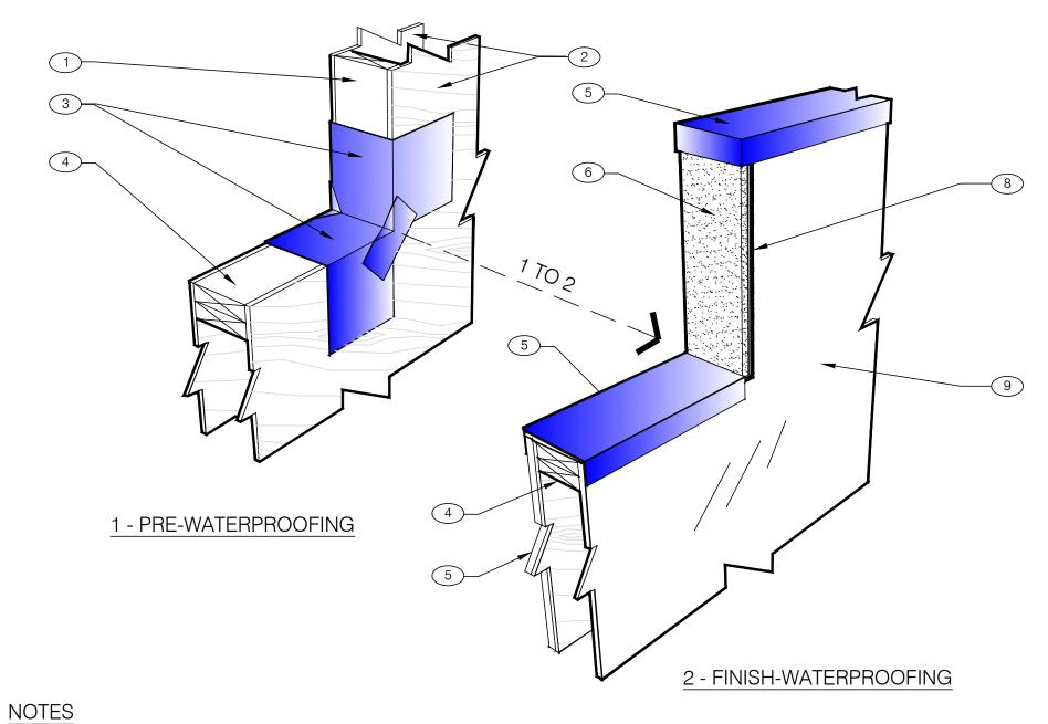
WRAP 1" THICK EIFS ONTO VERTICAL FACE OF PARAPET TRANSITION
