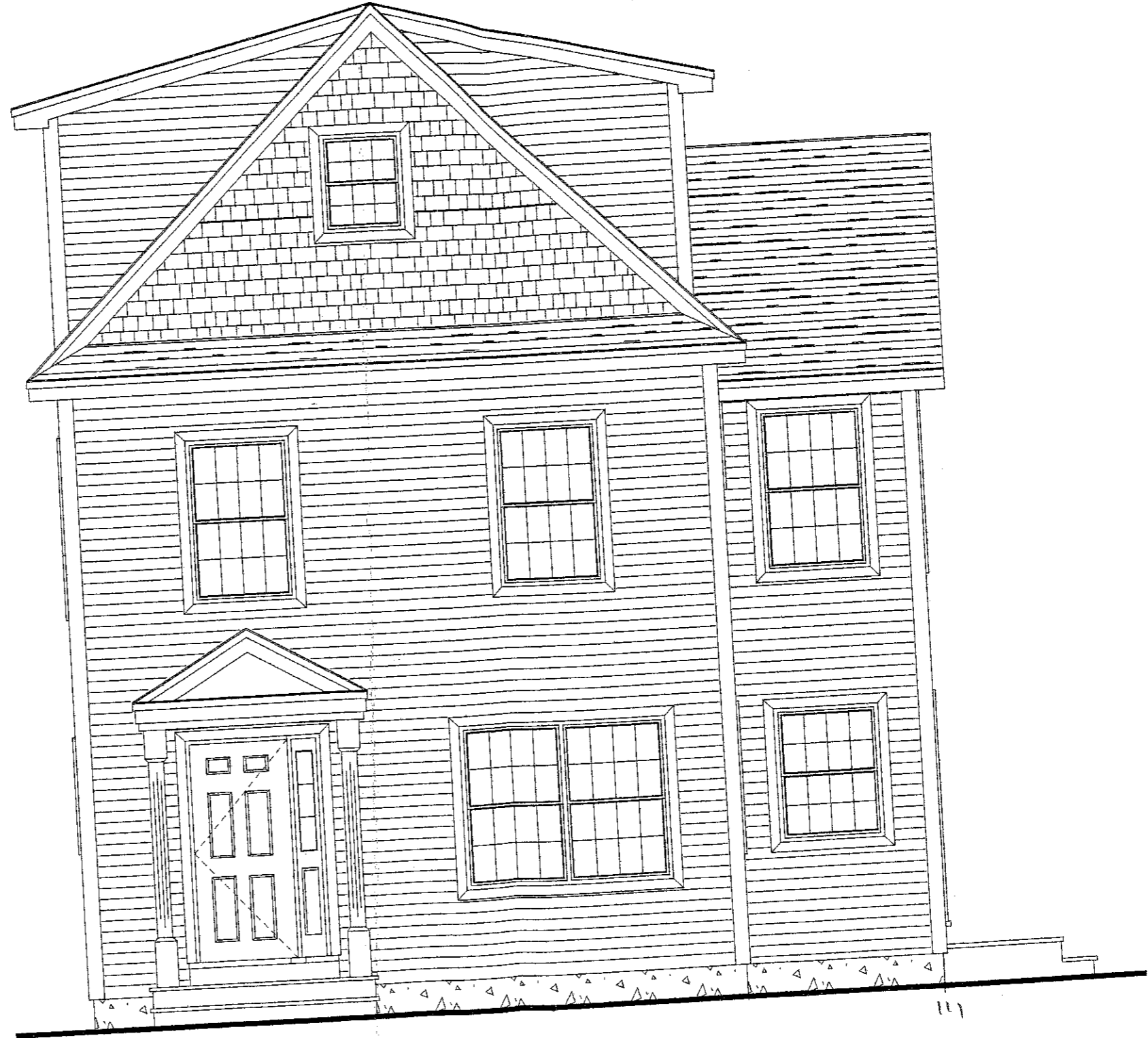
FRONT ELEVATION SCALE: 1/4" = 1'-0"
