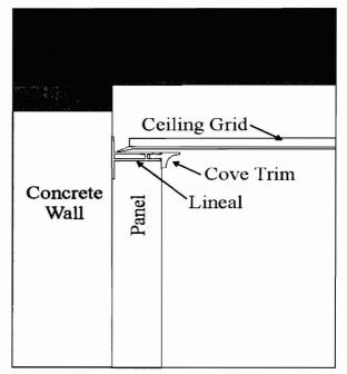
Hint: When installing a Mohave tile ceiling, save yourself some time by raising the grid system slightly off of the ceiling lineal / wall angle so you do not have to cut a reveal edge around the perimeter of the room! Pictured here are two ways of raising the grid, using pliers to bend the corners down at 45 degree angles or by attaching a 3/16" thick cabinet door bumper.
