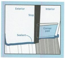
flap away from the frame and position the wedge behind the weatherstrip and against the sill so that the thin edge faces the edge of the door as it swings closed. Remove the backing paper and stick the wedge to the frame. Apply a bead of sealant at the intersection of the jambs, brickmoulds, thresholds and floor as shown.
