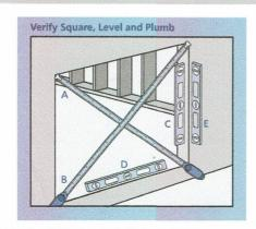
· Verify the rough opening is plumb (C, E and D). The maximum allowable deviation is 1/8".
