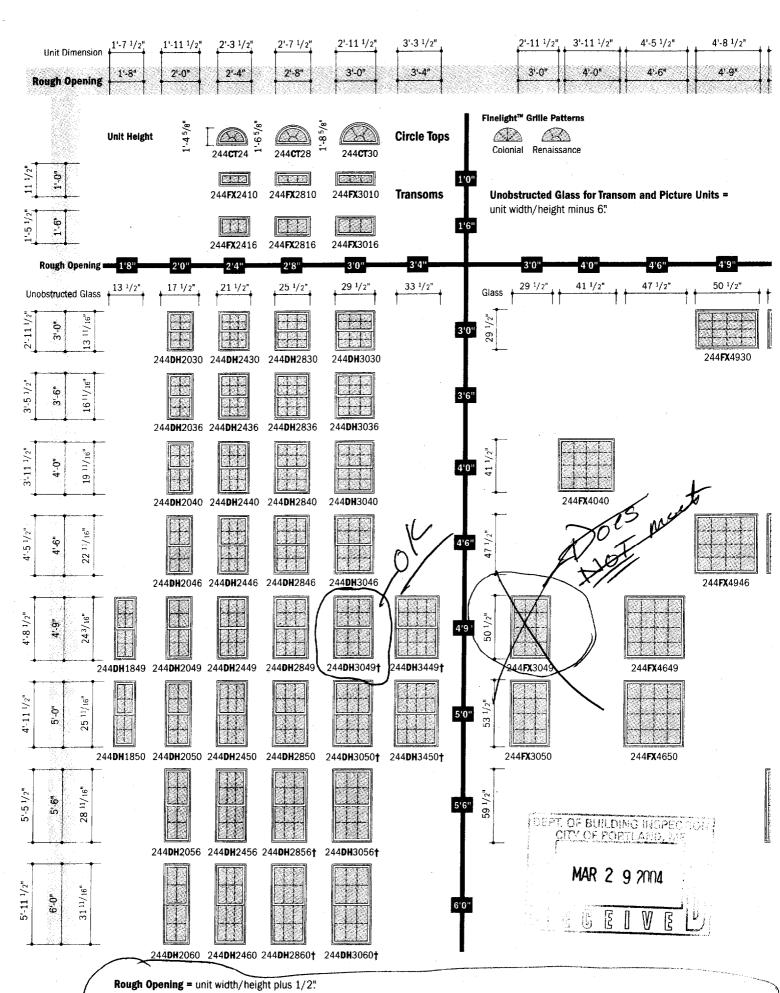
+ These units meet or exceed the following dimensions: clear openable area of 5.7 so. ft. clear openable width of 20° and clear openable height of 24°.
