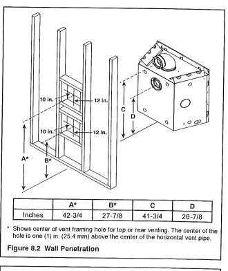
**Note:** When terminating horizontally off the top of the unit using SLP pipe, a 10 in. x 10 in. framing hole is required.
