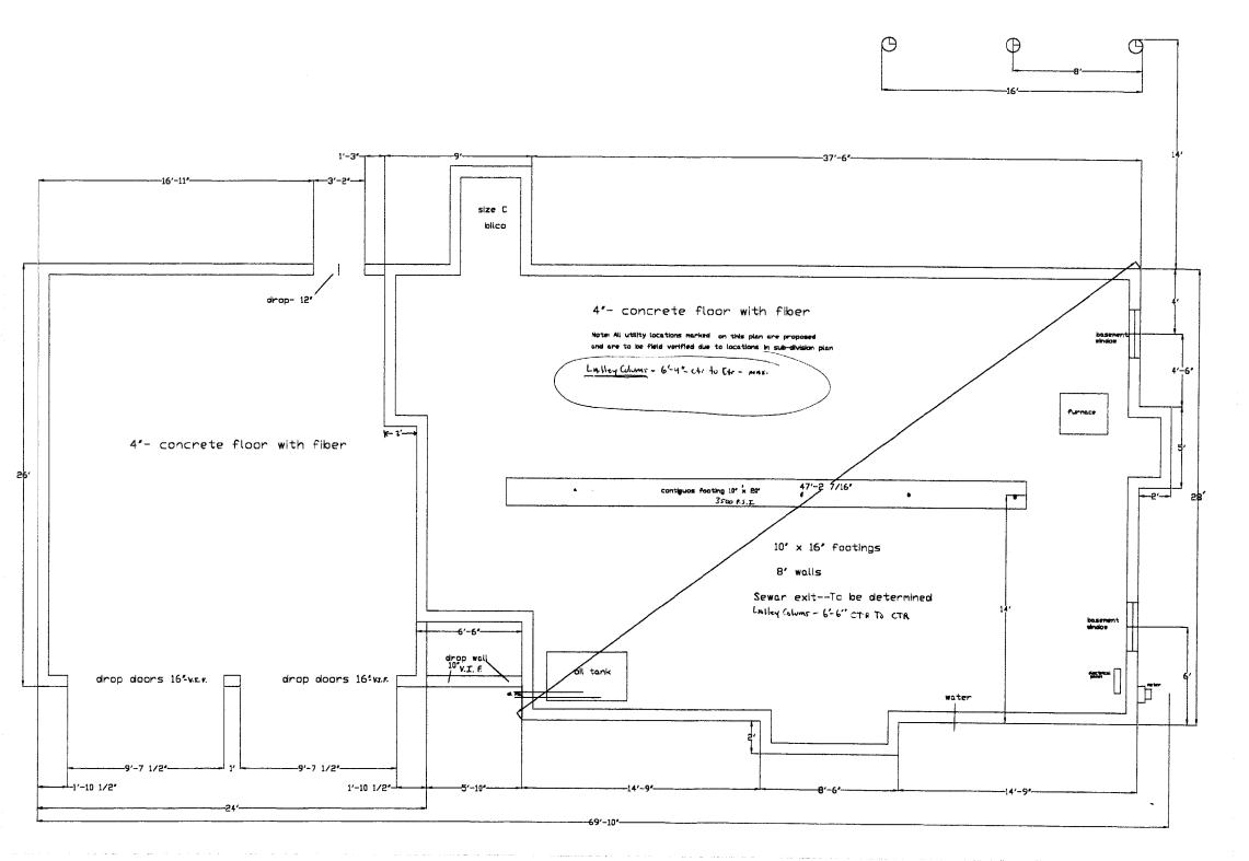
Note: Found after draways shall be Interior + Exterior Perimeter drains, crusted stone and perfected pipe, Foundation walls shall be plugged and Threed, Crushed stone shall be covered with filter Gabric, Sandfill against house walls.
