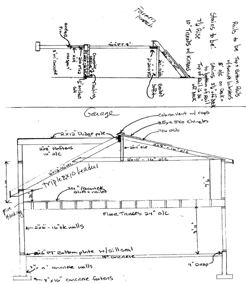
Sama tube for Bear Deck to be 4' tapened prefats concrete post w/ 7'6" max spacing! 10' out from building 2×8@160.C.
