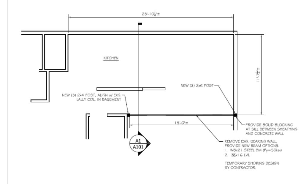
FIRST FLOOR PLAN w/ NEW BEAM TO SUPPORT 2nd FLOOR JOISTS
